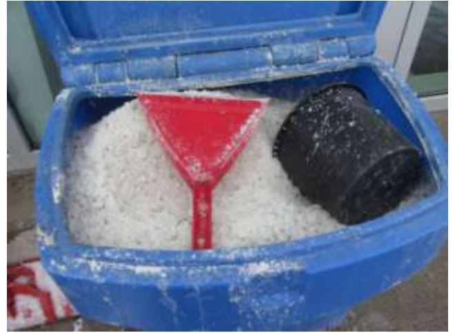
Inside the bin - no device to calibrate salt application
